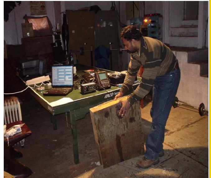
Trial testing of sandwiched plywood panel by ultrasonic amplitude analysis
